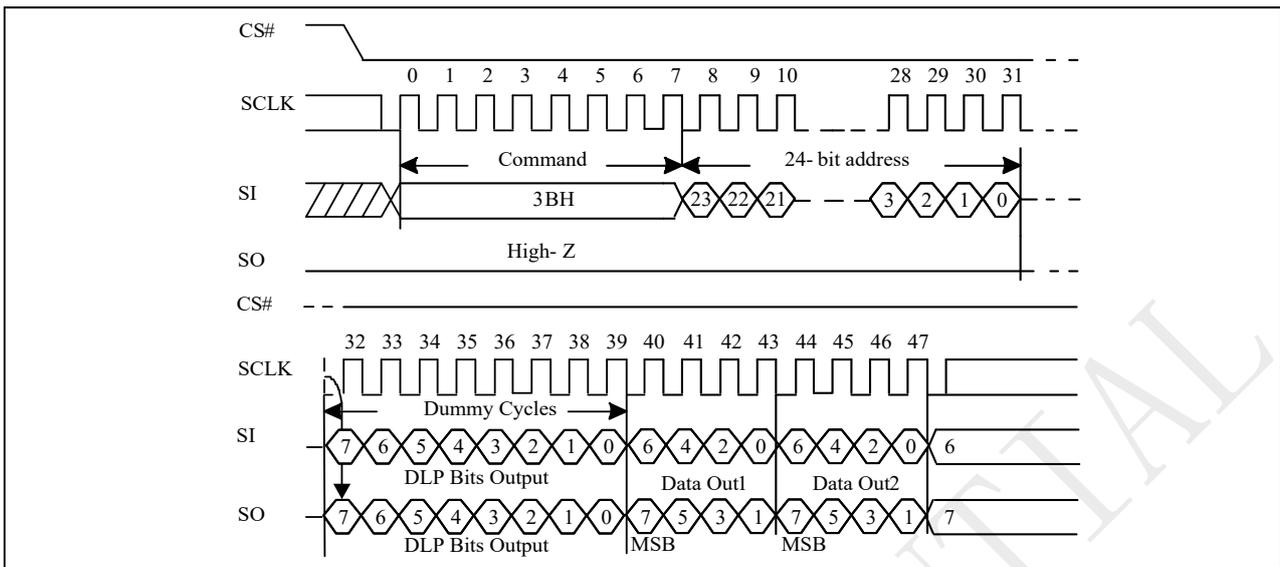
**Figure 10-23c 2IO Read with DLP bits output Sequence**
