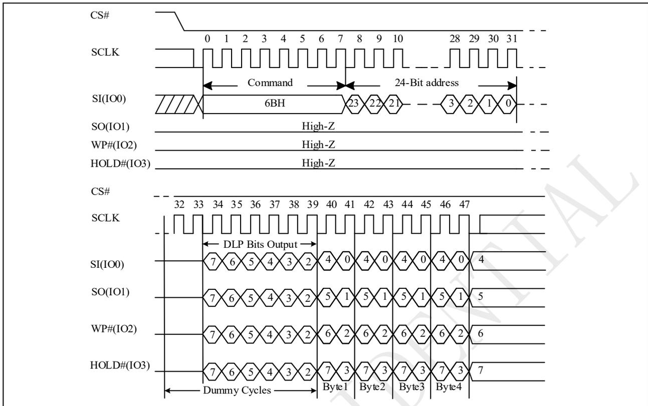
**Figure 10-23e 4IO Read with DLP bits output Sequence**
