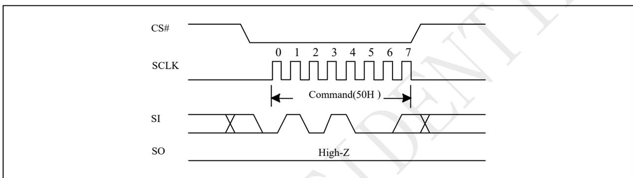
**Figure 10-4a Write Enable for Volatile Register Sequence (QPI)**
