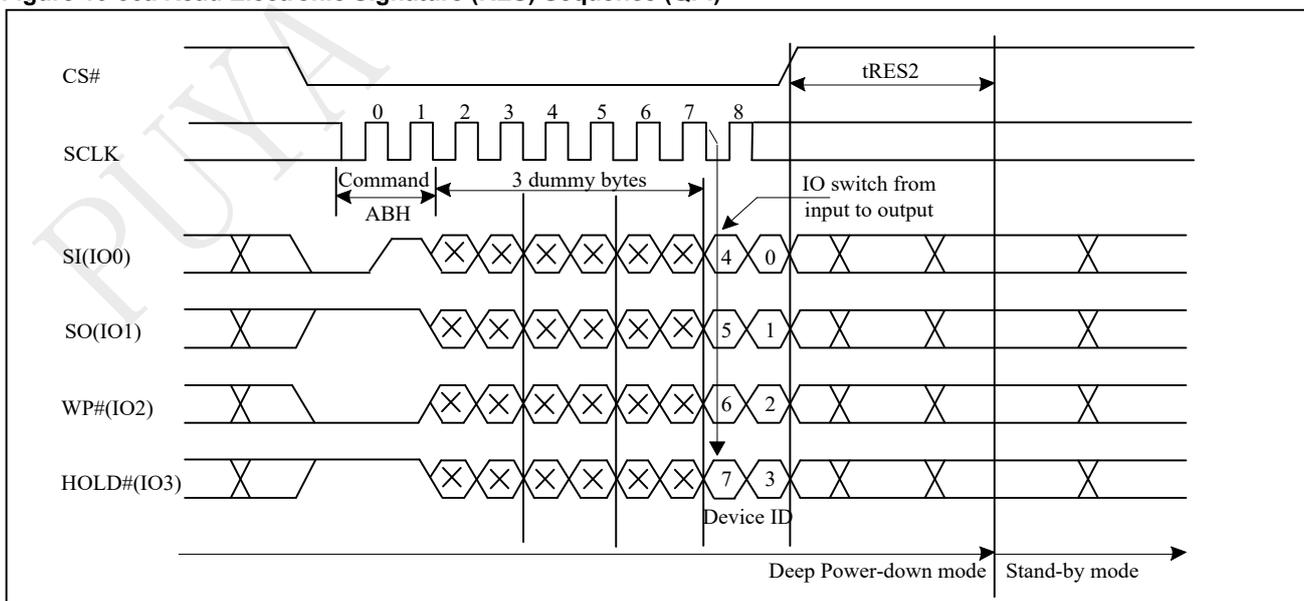
**Figure 10-36b Release from Deep Power-down (RDP) Sequence (Command ABh)**
