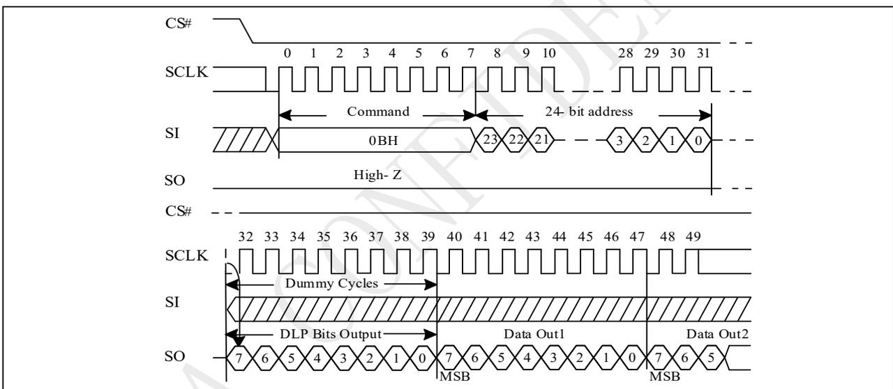
**Figure 10-23a Fast Read with DLP bits output Sequence in QPI mode**
