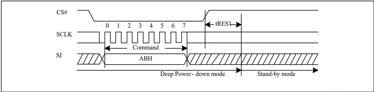
**Figure 10-36c Release from Deep Power-down (RDP) Sequence (QPI)**
