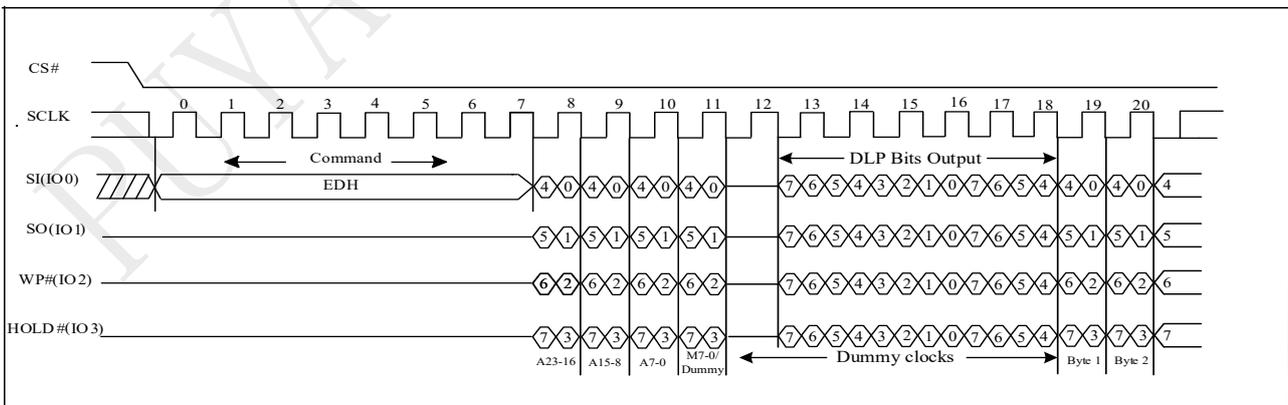
**Figure 10-23m DTR 4IO Read with DLP bits output Sequence in QPI mode**
