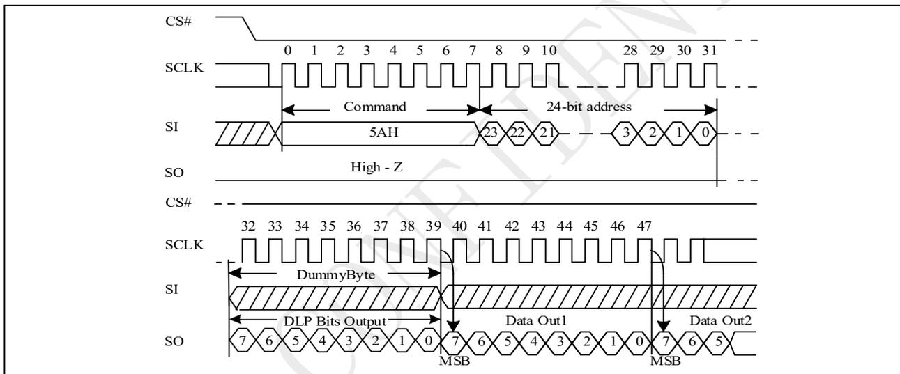
**Figure 10-23r Read Serial Flash Discoverable Parameter with DLP bits output Sequence in QPI mode**
