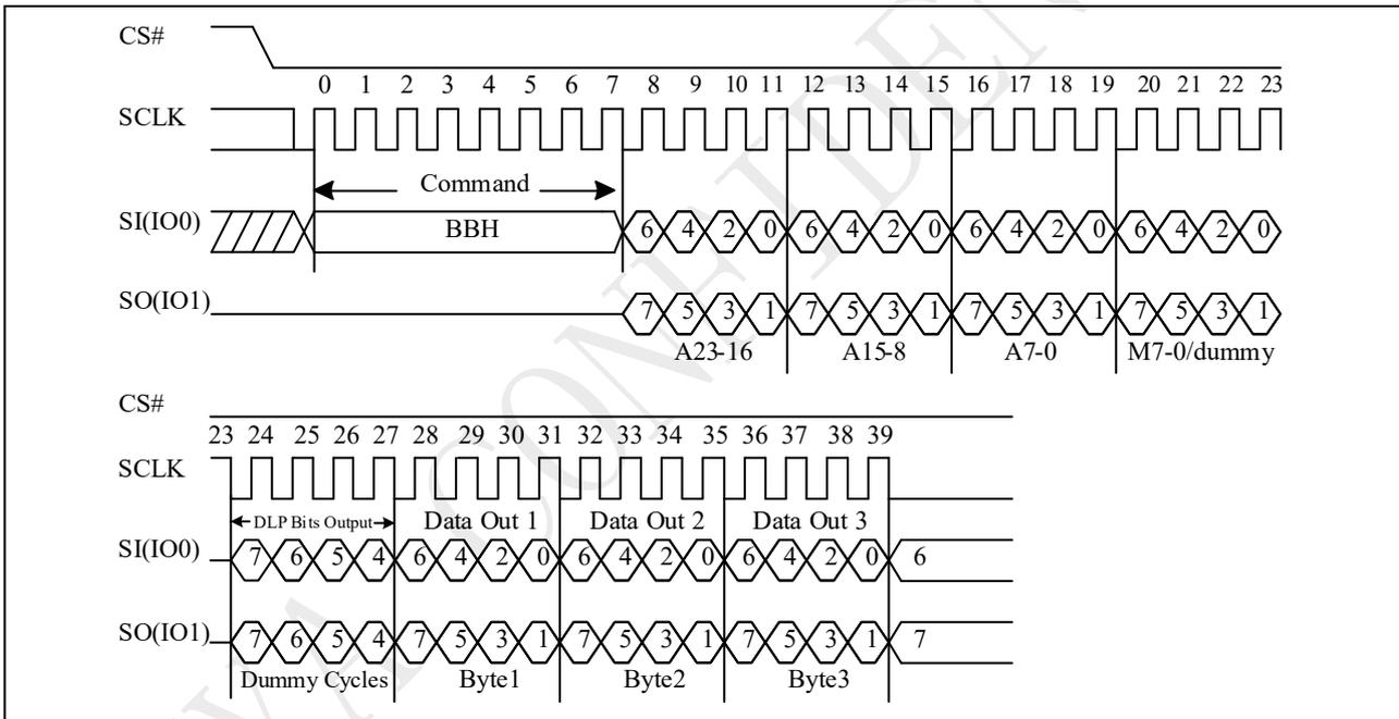
**Figure 10-23d Quad Read with DLP bits output Sequence**
